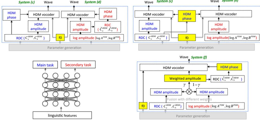
Figure 2: Left: Multi-task learning flowchart for INT (Multi-INT: system (c)) and DIR (Multi-DIR: system (d));  $f_0$  (yellow) is shared by both systems; Right top: Fusion of phase for multi-task learning (Multi-DIR-Phase: system (e));  $f_0$  and phase are shared (yellow part) by the two systems; Right bottom: Fusion of amplitudes for multi-task learning (Multi-Fusion: system (f))
