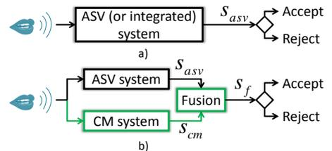
Figure 1: Traditional way to protect automatic speaker verification (ASV) from spoofing attacks is to independently develop ASV and countermeasure (CM) subsystems that are post-combined with score-level fusion (b). Our core contribution is a *joint* approach that uses same i-vectors for both speaker verification and voice conversion attack detection.  $s_x$  means a score produced by system  $x$ .
